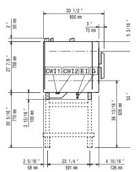
CWII Cold Water inlet 1 Cold Water Inlet 2 CWI2
